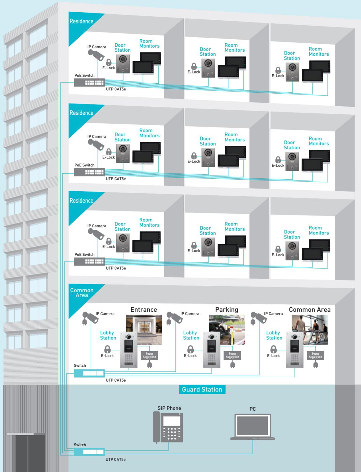
Support up to 2,000 devices on a system with a Control Box
